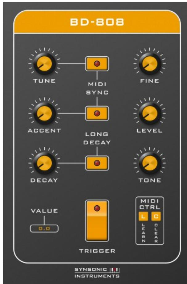
The Synsonic-Instruments BD-808 plugin is a model of the original bass drum circuit of the famous Roland TR-808. A very detailed analysis of the electrical circuit behaviour and the special effects of the analog parts results in an authentic sounding virtual analog bass drum plugin. Especially for genres like Techno and Hip-Hop this kind of bass drum sound can be interesting. We hope you will have fun with it!
